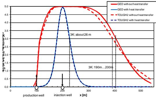
Figure 5: Cross section through the „plume“ of test 2 after 30 years of operation without (analog to Figure 4) and with heat transfer (blue).
