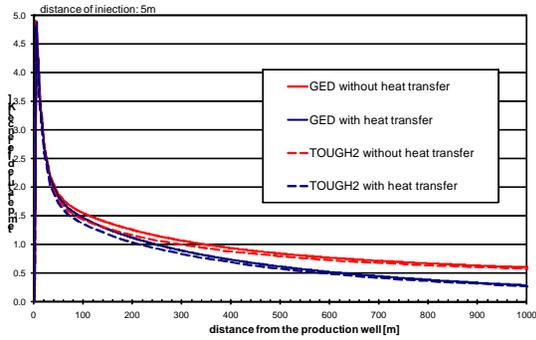
Figure 3: Temperature profile through the „plume“ of test 1 after 30 years of operation without (analog to Figure 2 bottom) and with heat transfer (blue).
