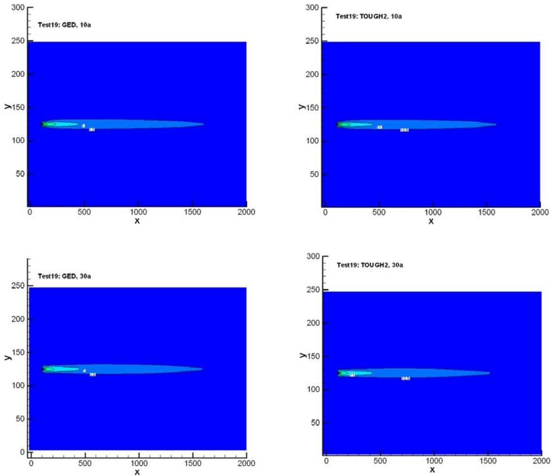
Figure 2: Detail of results: left GED, right TOUGH2, on top after 10 years, on bottom after 30 years of operation [dark blue: unaffected temperatures; isotherms of 0.5K and 1K change indicated<sup>1</sup>].
